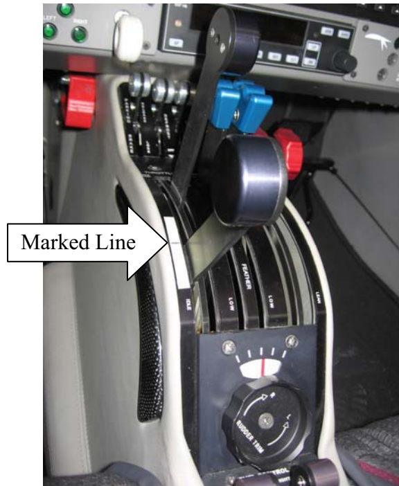
Figure 205 - Marking the Front Edge of the Throttle Lever
