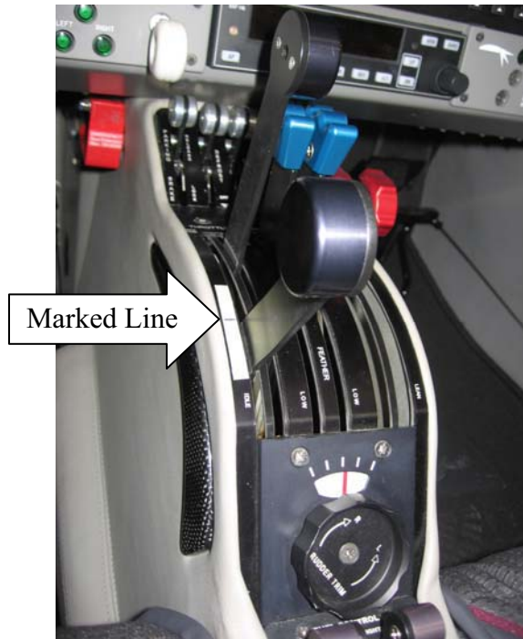
Figure 203 - Marking the Front Edge of the Throttle Lever
