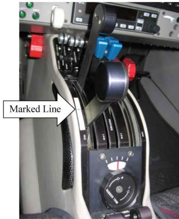
Figure 206 - Marking the Front Edge of the Throttle Lever
